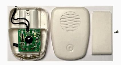
Close the housing, hook into the top where the antenna is and press together. Tighten the screw.
